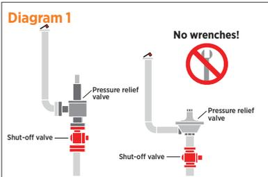
Do not attempt to close a shut-off valve on a meter set that includes a pressure relief valve. Shut-off valves on these meter sets are typically locked and should remain open. **(Dia 1)**
